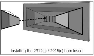
Reinstall the grille by placing one side of the grille under the side cleat, then gripping the grille on the top and bottom, bend the other end under the cleat at the opposite end of the cabinet. With the inserts installed, the horizontal coverage angle is reduced to  $60^{\circ}$ .
